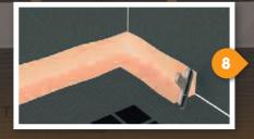
Seal all joints (both wall and floor) utilising special waterproof membrane / paste.
