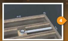
Fix a batten below the top of the joists.
